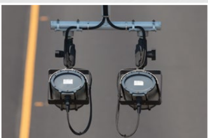
Violation enforcement cameras allow for billing of those that use the express lane even if they travel without a FasTrak transponder.
