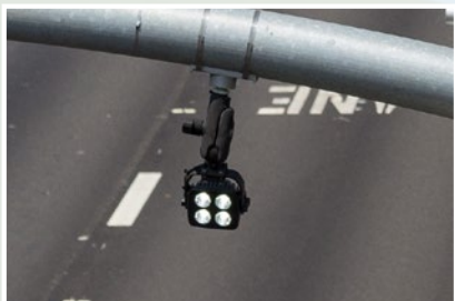
LED lights are used to illuminate the license plate capture cameras.
