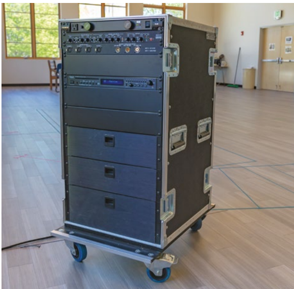
PCD installed Anvil Racks in each of the 3 rehearsal rooms. The racks contain an amplifier, mini mixing console, Whirlwind mixer and a Denon Pro CD player.
