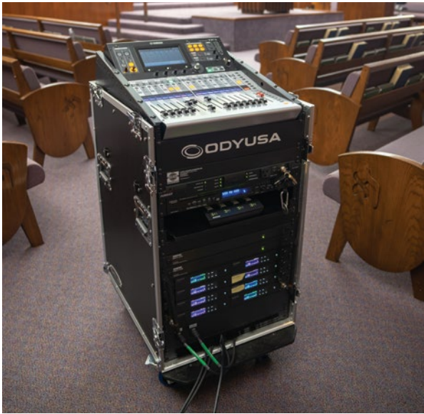
A Yamaha digital mixer sits on a portable rack, allowing the Temple's audio engineers to easily calibrate the new sound system during performances.
