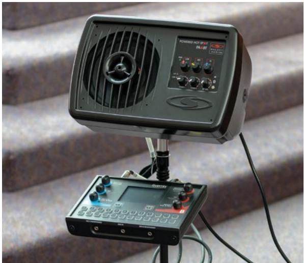
A PA6BT Powered Hot Spot Personal Monitor was installed to provide the Temple's musicians a personal active compact monitor.
