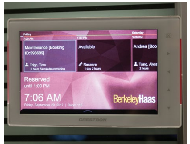
All of the rooms in the building contain a Crestron controller which displays when the room is available or scheduled to be used.
