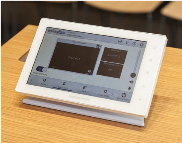
The event space Primeview LED video wall is controlled through a Crestron touch panel.
