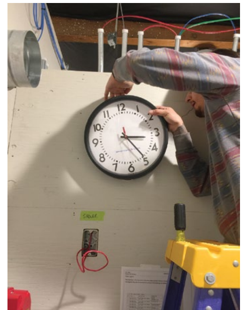
Students learn how a wireless analog battery clock synchronizes to the radio signal transmitted from the wireless master, making sure it is operating properly.
